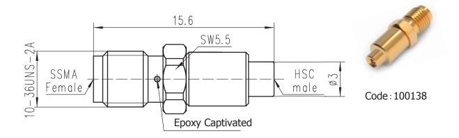
This part can be used to test wireless system, such as Mobile phone, Wireless LAN, mini-PCI, Bluetooth, PDA, GPS etc.. It match with Murata HSC series receptacles.
