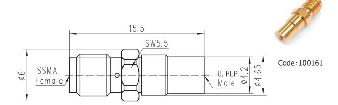
This part can be used to test wireless system, such as Mobile phone, Wireless LAN, mini-PCI, Bluetooth, PDA, GPS etc.. It match with Hirose U.FL series, I-PEX 20431 and Amphenol AMC series etc. receptacles.
