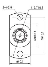
This part can be used to test wireless system, such as Mobile phone, Wireless LAN, mini-PCI, Bluetooth, PDA, GPS etc.. The inner PIN or outer contact of probe is sharp, so it's suitable to test for PCB PAD.
